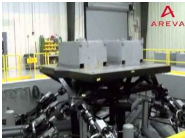
Figure 57: AREVA's seismic shake table with three orthogonal vibratory motion, (from us.aveva.com )
